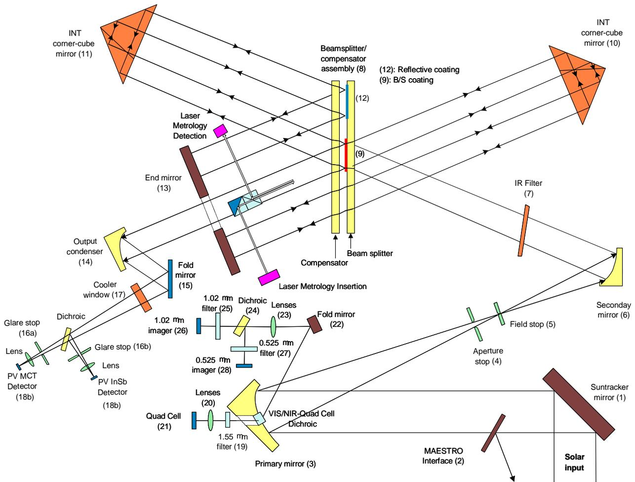
Figure 2: ACE-FTS instrument optical layout
