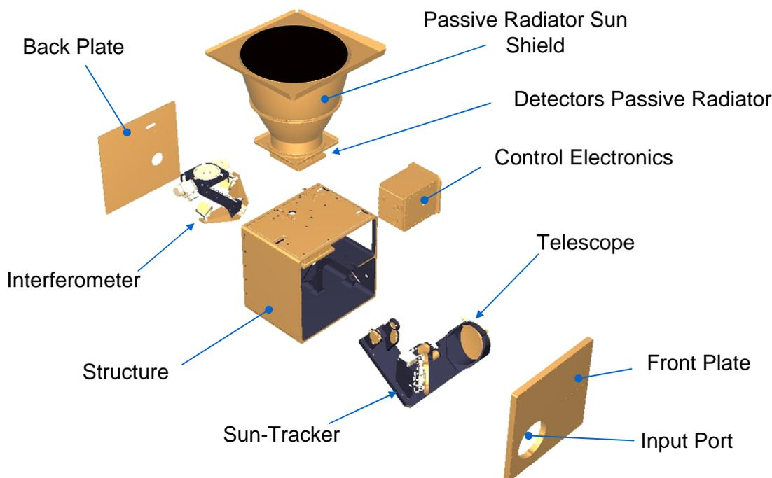
Figure 3: Exploded 3-D view of the ACE-FTS
