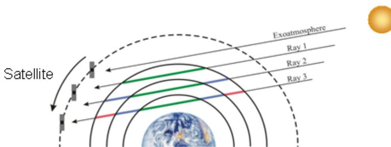
Figure 1: Solar Occultation Principle around the Earth
