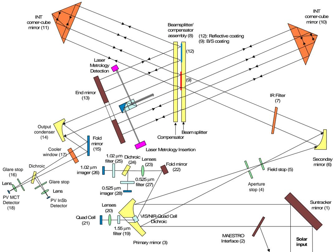
Figure 1: ACE-FTS instrument optical layout
