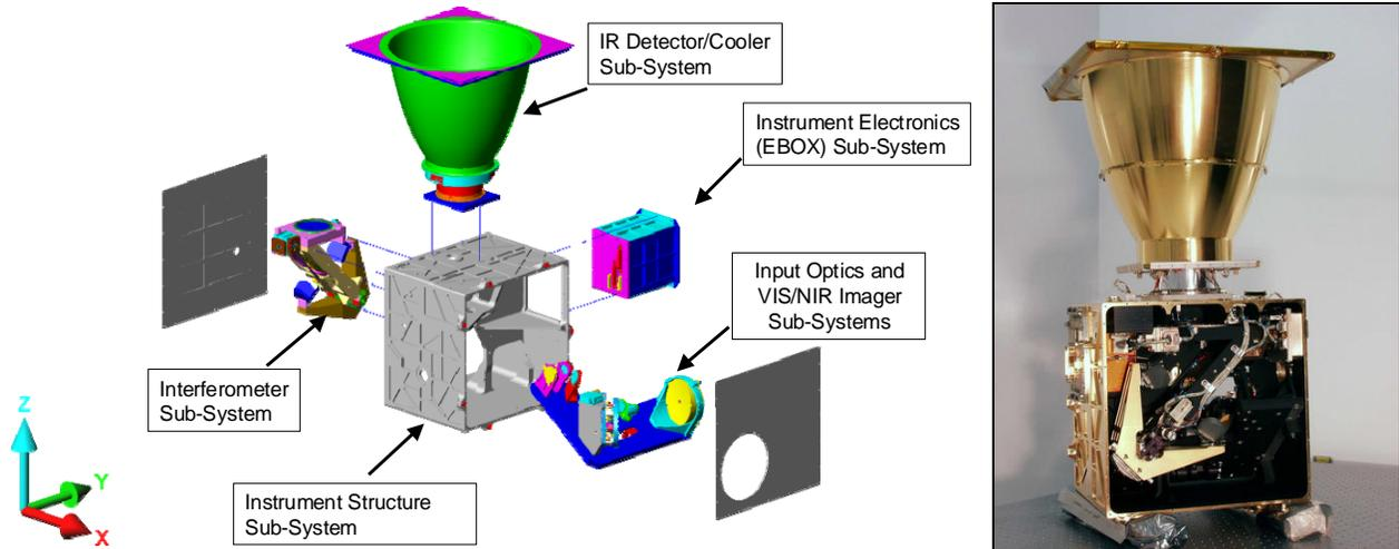
Figure 2: ACE-FTS architecture (left) and picture of the Flight Model (right)
