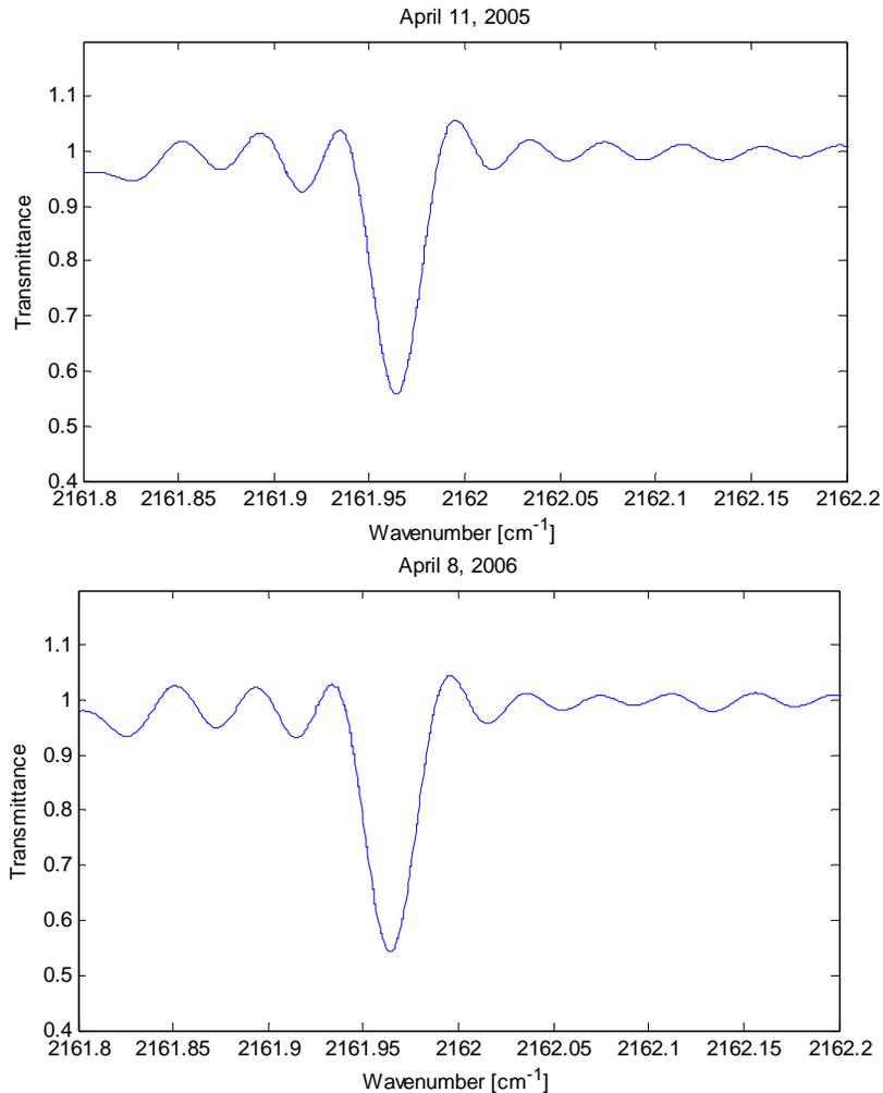
Figure 8: On-orbit FTS instrument line shape taken
