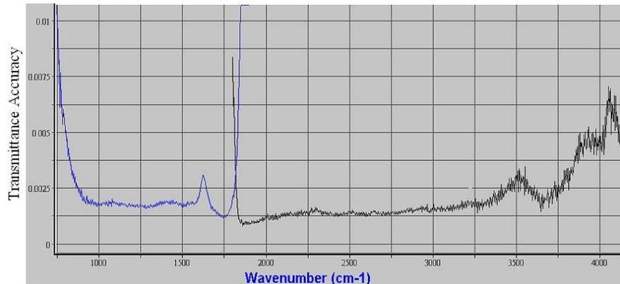
Figure 7: On-orbit FTS transmittance accuracy
