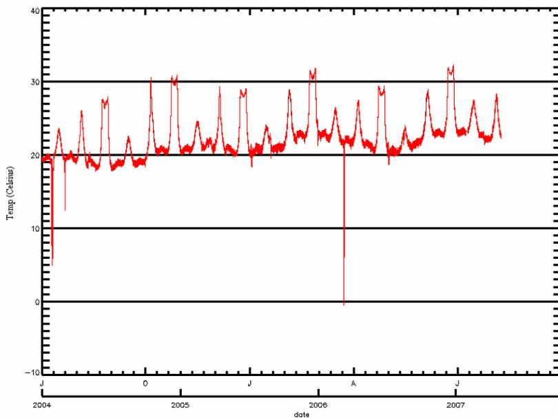
Figure 9: On-orbit FTS temperature (interferometer beamsplitter) 2004-2007
