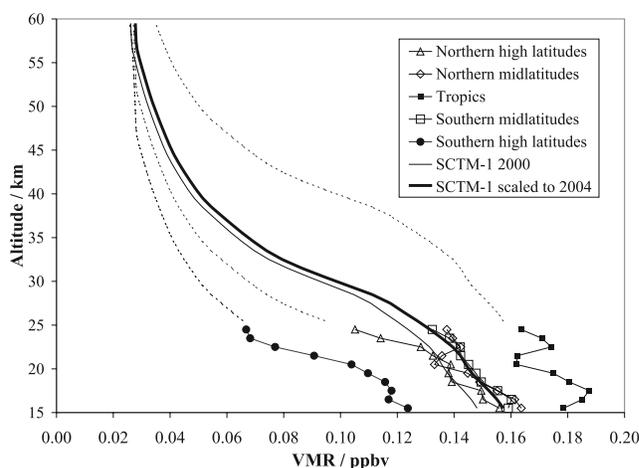
**Figure 2.** Profiles of  $\text{CHClF}_2$  (HCFC-22) in the stratosphere: the SCTM-1 modeled profile for  $45^\circ\text{N}$  in 2000, the SCTM-1 profile scaled for 2004, and ACE-FTS measured values in the northern high latitudes, northern midlatitudes, tropics, southern midlatitudes, and southern high latitudes. The scaled and shifted SCTM-1 profiles for extending the ACE-FTS measurements to higher altitudes are shown as dotted lines.
