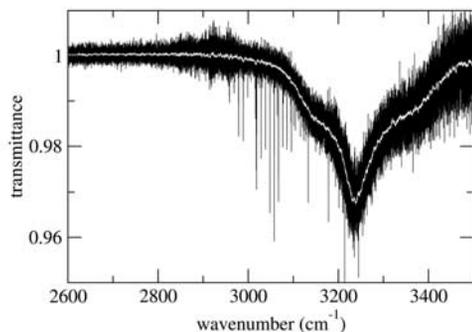
**Figure 5.** PMC absorption in ACE-FTS spectra. The O-H stretch feature is evident in this average of 9 spectra (black) taken during 6–14 July 2004, near 66°N. All spectra have tangent point altitudes near 83 km. The result of a 128-point median filter is shown as the white line. This feature is consistent with absorption by ice particles with  $\sim 50$  nm effective radius.
