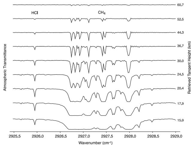
**Figure 2.** A small section of spectra from ACE-FTS. The R(0) line of the HCl fundamental band on the left and the cluster of CH<sub>4</sub> lines due to R(9) of the  $\nu_3$  band on the right. The retrieved tangent heights (in km) are on the right side.
