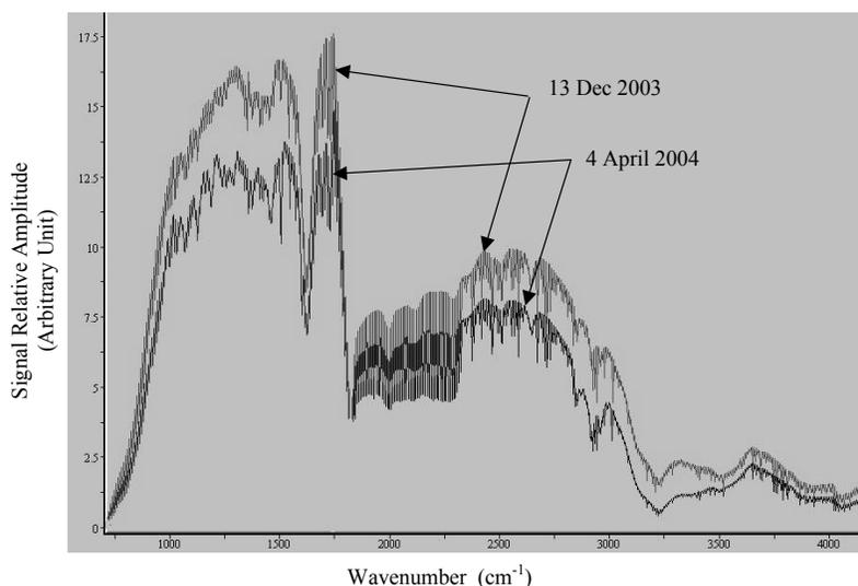
Figure 3. IR signal amplitude right after the second full decontamination and four months later (without additional full decontamination)
