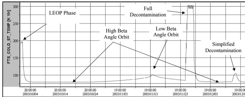
Figure 9. On-orbit IR detectors cryo-cooler thermal profile
