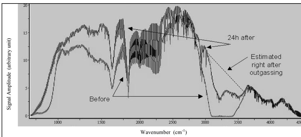
Figure 1. Signal amplitude of the IR channels before (lower curve) and 24 hours after cryo-cooler decontamination (upper curve)
