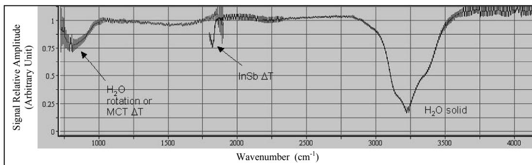
Figure 2. Ratio of the IR signal taken 5 days after simplified decontamination over the signal measured just after simplified decontamination
