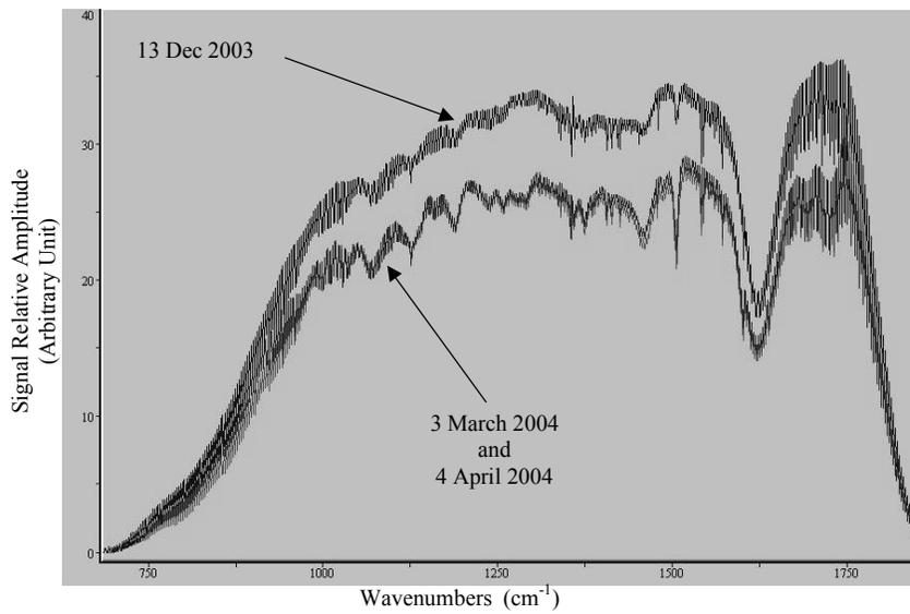
Figure 4. IR signal amplitude (long wave channel) right after, three months after, and four months after full decontamination
