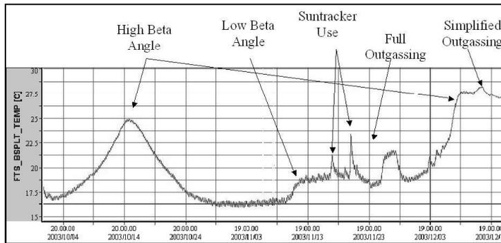
Figure 8. On-orbit ACE-FTS instrument thermal profile
