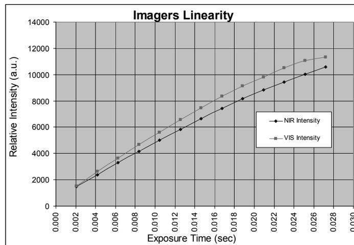
Figure 5. Imagers response vs. exposure time
