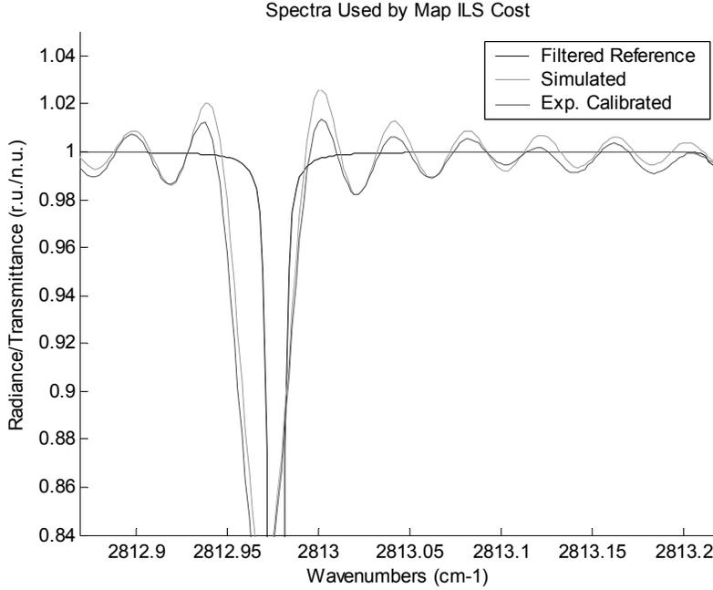
Figure 7: Measured and fitted N<sub>2</sub>O absorption line for a half divergence inside the interferometer of 5.1 mrad offset from the optical axis by 1.28 mrad.
