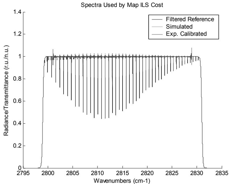
Figure 5: Simulated and experimental spectra for nominal ILS distortion. The cost value is 3.285.
