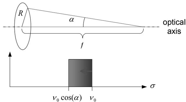
Figure 2: Off-axis effect and line broadening impact
