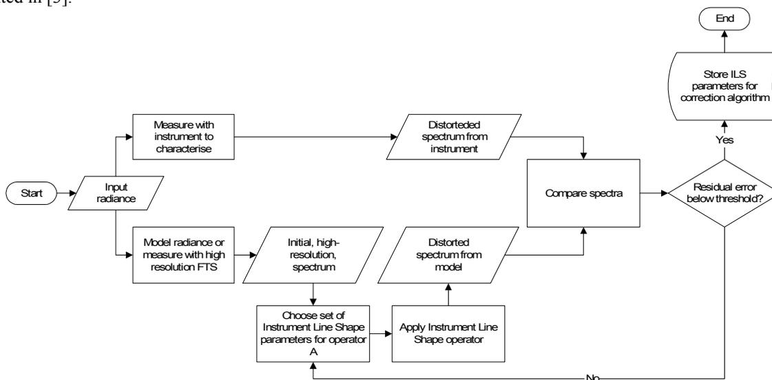
Figure 3: Instrument line shape characterisation flow diagram.
