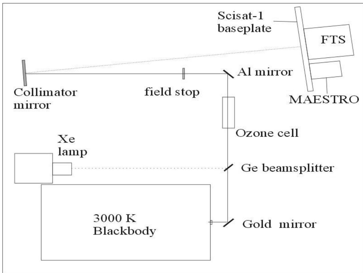
Figure 1: Schematic diagram of the testing configuration used for the ozone measurements with the ACE FTS and MAESTRO instruments. The germanium beamsplitter serves to combine the ultraviolet light of the xenon source with the visible light of the high-temperature blackbody radiator.
