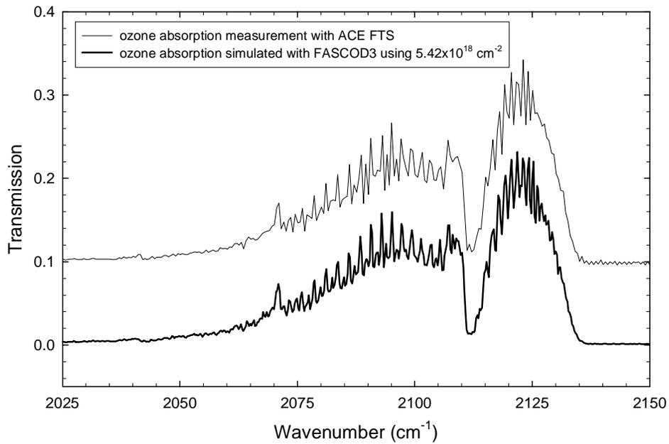
Figure 6: The transmission spectra of ozone as measured with the ACE FTS and simulated with the FASCOD3 model. The comparison of the band integrals for the measurement and simulation shows that 200 DU ( $5.42 \times 10^{18}$  molecules/cm<sup>2</sup>) of ozone was present in the gas cell. This evaluation compares favourably with the average result of  $6.16 \times 10^{18}$  cm<sup>-2</sup> that was determined from the measurements made with the Magna FTS.
