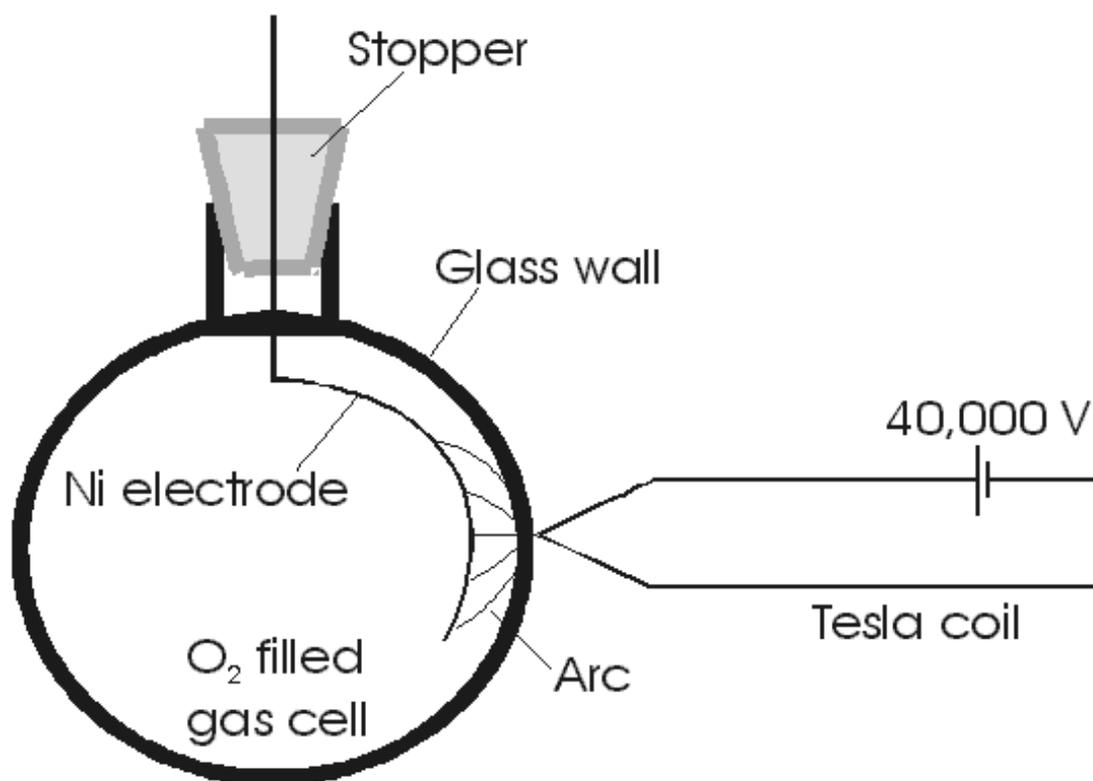
Figure 2: Schematic diagram showing the end-view of the gas cell set up for generating ozone.
