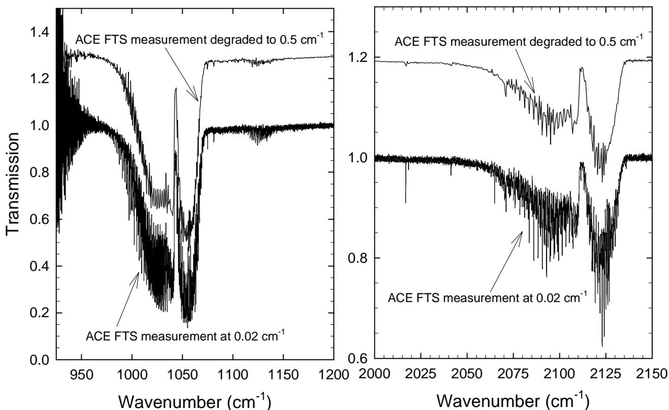
Figure 5: The transmission spectra of the ozone gas cell measured with the ACE FTS at a high resolution of  $0.02\text{ cm}^{-1}$ . Also shown are the spectra degraded to a resolution of  $0.5\text{ cm}^{-1}$  for the purpose of determining the column amount of ozone in the cell (see Figure 6).
