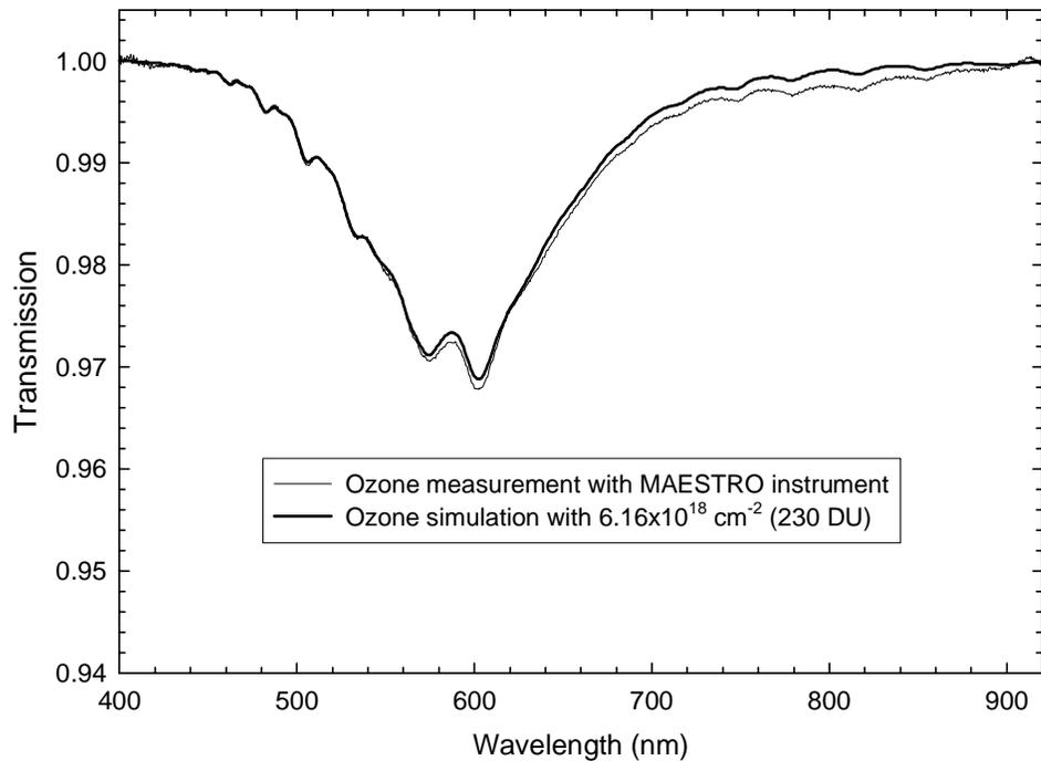
Figure 7: The transmission spectra of ozone measured with the MAESTRO instrument and simulated with the MODTRAN4 model. An amount of  $6.16 \times 10^{18}$  cm<sup>-2</sup> of ozone was used in the simulation. This was based on the ozone amount determined from the average of the Magna FTS results.
