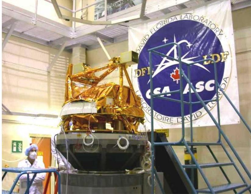
Figure 4: ACE-FTS Vibration test Qualification at Spacecraft Level.
