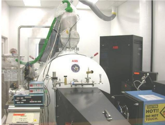
Figure 10: ACE-FTS TVAC Qualification at Instrument Level.
